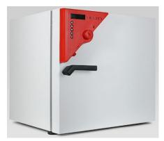
All the ovens are fitted with an over temperature safety cut-off switch to Class 2 (DIN 12880).
